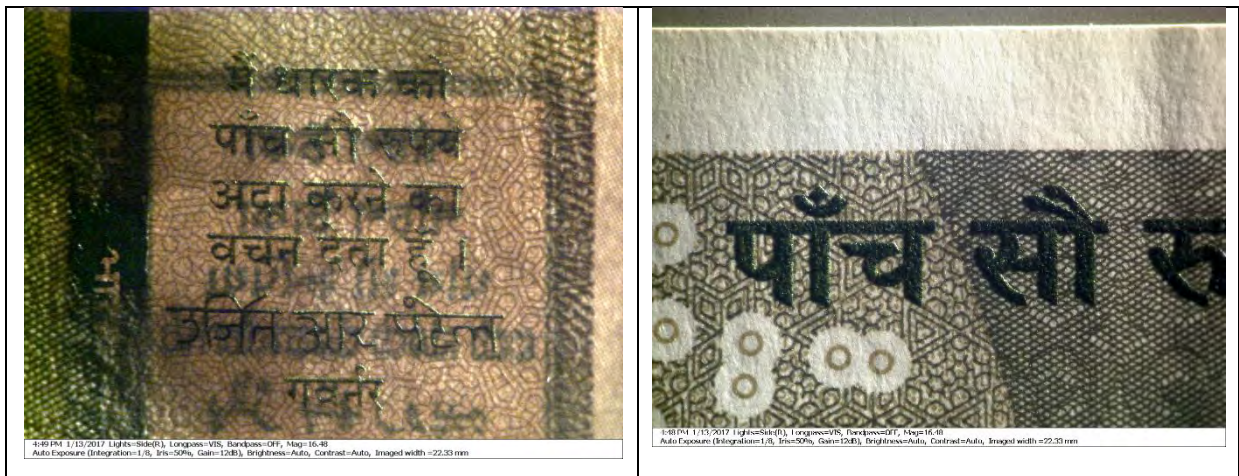
Figure 20: Paper currency note of ₹ 500, Promise clause and other writings is printed by Intaglio printing
