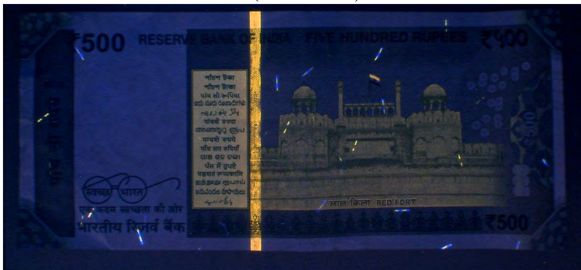
5:30 PM 1/5/2017 Lights=365nm Ultra Violet, Longpass=VIS, Bandpass=OFF, Mag=2.077 Integration=2 Sec, Iris=50%, Gain=12dB, Brightness=50, Contrast=30, Imaged width =177.18 mm
