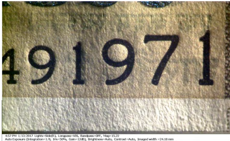
Figure 21: Paper currency note of ₹ 500, currency number is printed by Letter press printing.
