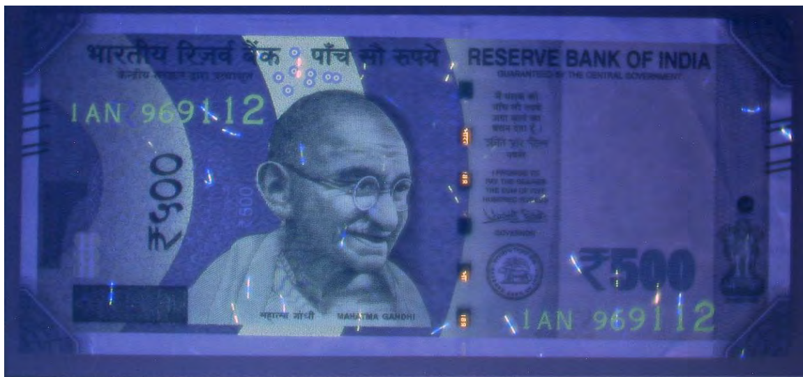
5:26 PM 1/5/2017 Lights=365nm Ultra Violet, Longpass=VIS, Bandpass=OFF, Mag=2.077 Integration=1.4 Sec, Iris=73%, Gain=12dB, Brightness=50, Contrast=30, Imaged width =177.18 mm
