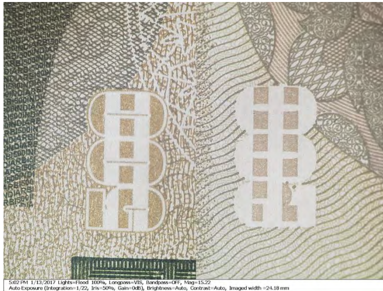
Figure 10: Paper currency note of ₹500 showing see through register denomination number 500 in transmitted light (both side comparable image).
