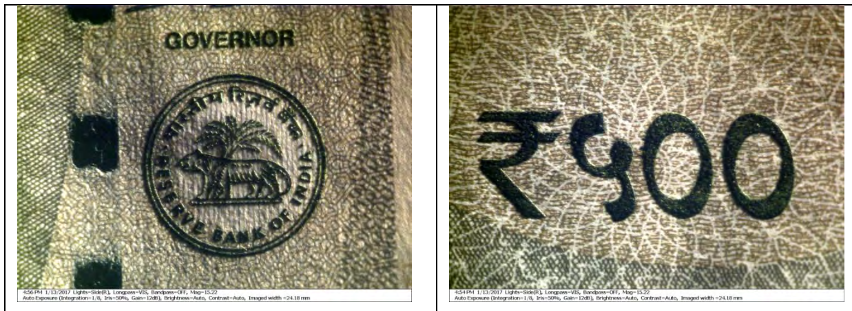
Figure 18: Paper currency note of ₹ 500, Reserve Bank of India seal, ₹ 500 is printed by Intaglio printing.
