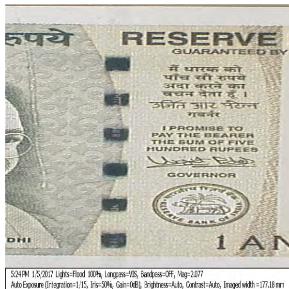
Figure 7: Paper currency note of ₹ 500 showing green colour security thread in visible light
