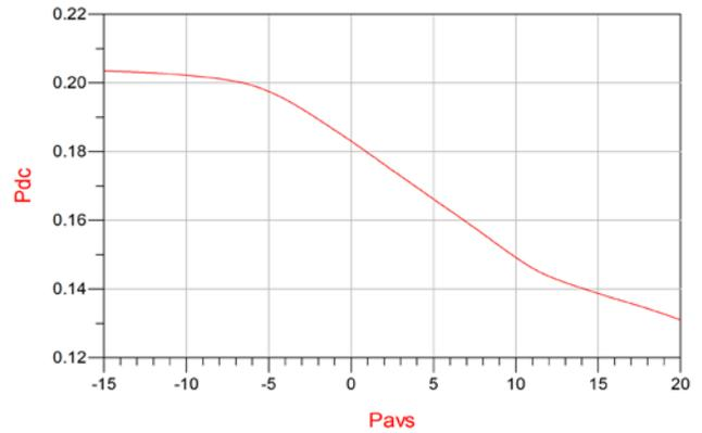
Fig.11 Simulated DC power consumption (Pdc) of the 60GHz power amplifier.
