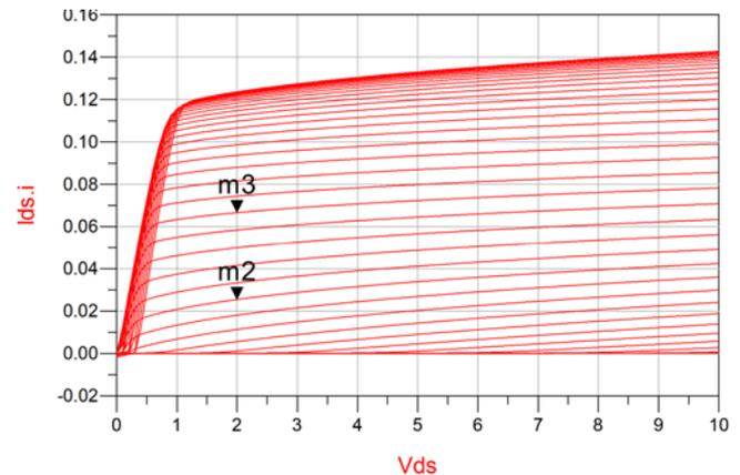
Fig.3 static characteristic Ids according to Vds for different Vgs values.
