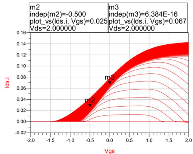
Fig.4 Ids according to Vgs for different Vds values.
