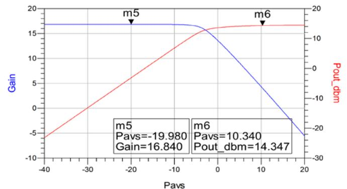
Fig.8 Plot of simulated Measured PA power gain and output power curves at 60 GHz.
