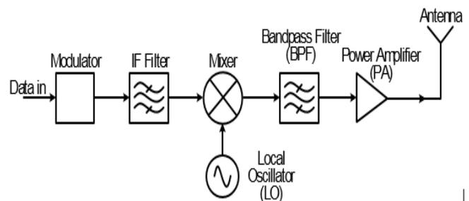
Fig.1 Block diagram of a basic RF transmitter (Tx)
