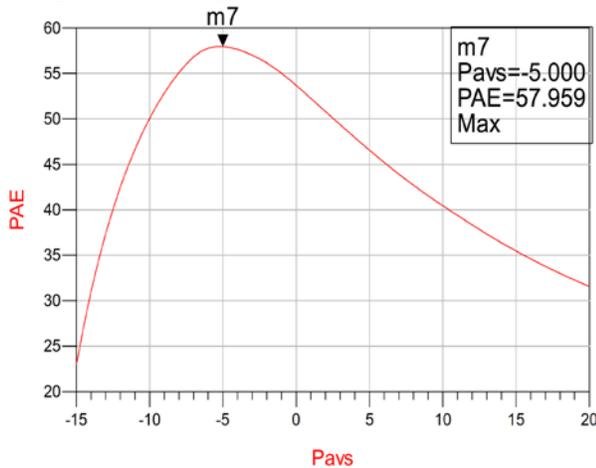
Fig.10 Simulated power added efficiency (PAE %) of the 60GHz power amplifier.
