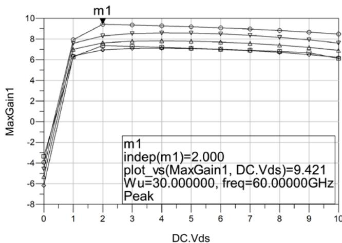
Fig.2 MaxGain as a function of Vds and Wu (Wu= 10 μm (□); Wu= 30 μm (○); Wu= 50 μm (▼); Wu= 70 μm (Δ); Wu= 90 μm (◇)).
