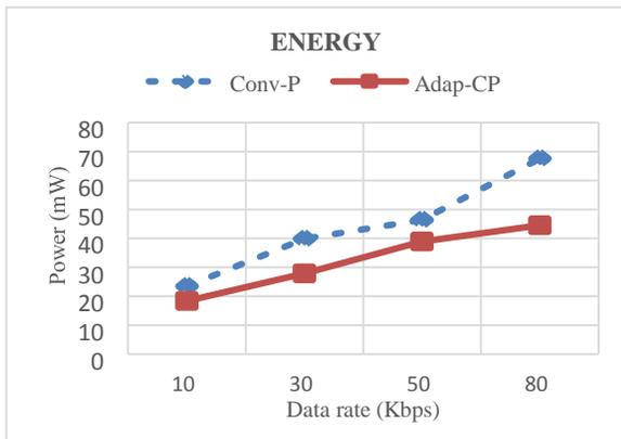
Figure 4. Energy consumption of Conv-P and Adap-CP for static network
