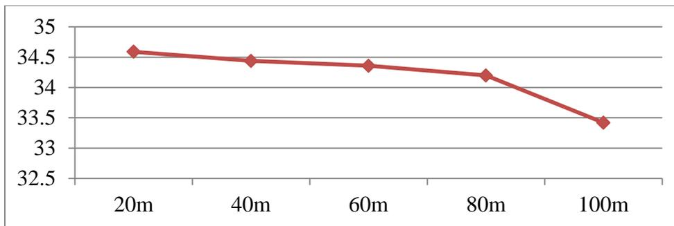
**Fig. 4.4** Power density against distance (9mobile Base station)
