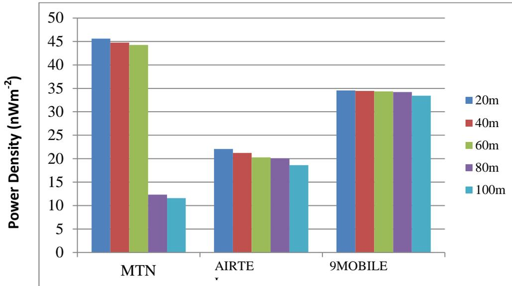
**Fig. 4. 1:** Power densities at different distances for tested base stations
