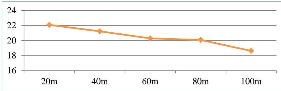
**Fig. 4.3** Power density against distance (Airtel Base station)
