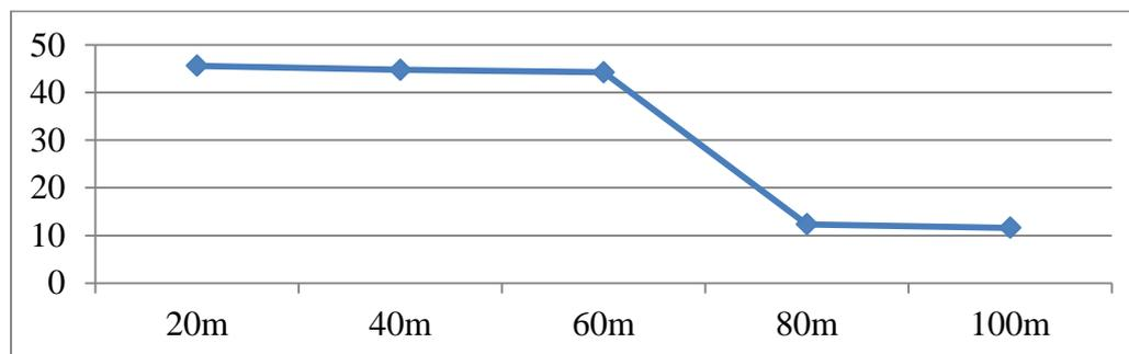
**Fig. 4.2** Power density against distance (MTN Base station)
