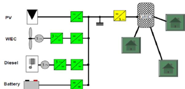
Fig.3 Schematic diagram of a PV mini-grid structure[6]
