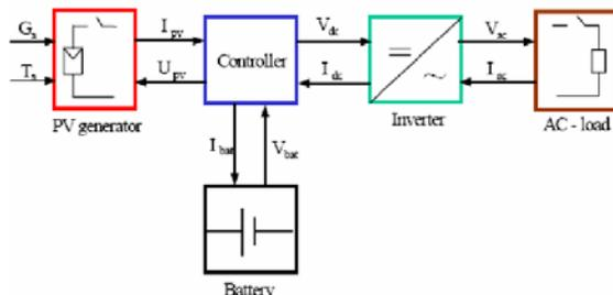
Fig.1 Block diagram for the standalone PV system[7]
