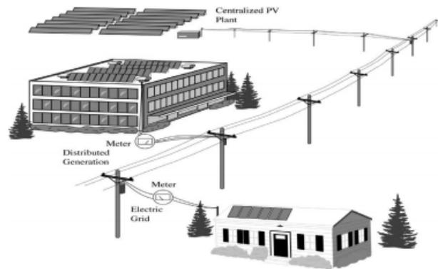
Fig.2 Schematic diagram of a PV mini-grid system[6]
