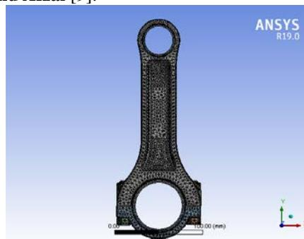
Figure 1.4: Tetrahedron mesh connecting rod
