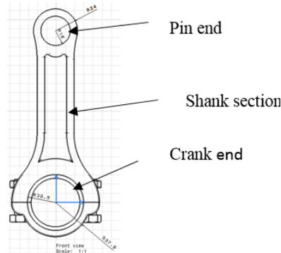
Figure 1.1: Schematic design of connecting rod.
