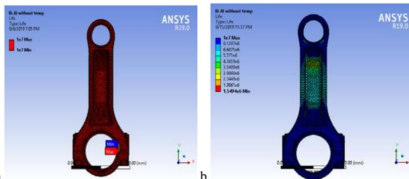
Figure 1.11: a. Fatigue life of aluminium alloy 7068, b. Fatigue life of aluminum alloy 7050T7651
