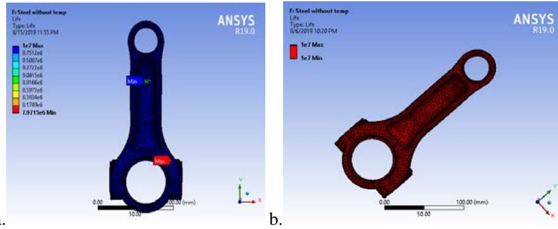
Figure 1.12: Fatigue life of carbon steel C-40, b. Fatigue life of forged Steel 4340
