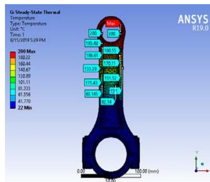
Figure 1.6: Temperature distribution on connecting rod
