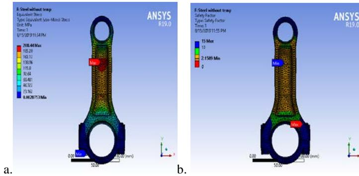
Figure 1.9: a. Von-mises stress, b. Safety factor
