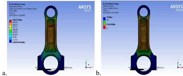
Figure 1.8: a. Von-mises stress, b. Safety factor
