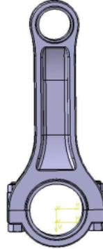
Figure 1.3: Assembly modeling of connecting rod
