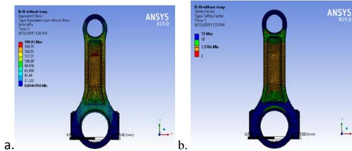
Figure 1.7: a. Von-mises stress, b. Safety factor
