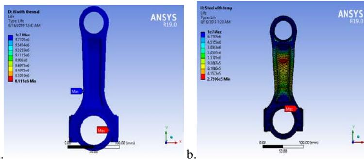
Figure 1.13: a. Fatigue life of Aluminum Alloy 7068 T6, b. Fatigue life of aluminum Alloy 7050T7651
