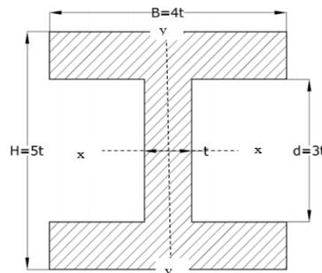
Figure 1.2: Configuration of I-Section connecting rod
