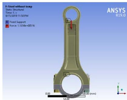
Figure 1.5: Boundary condition of the connecting rod
