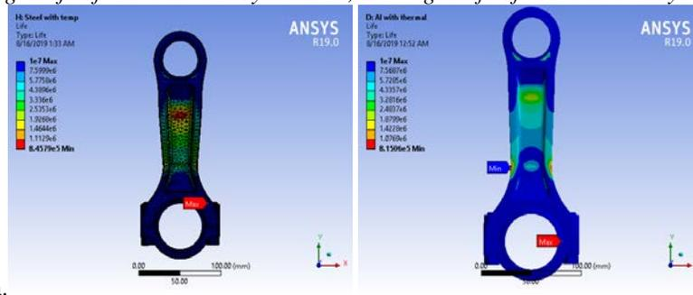
Figure 1.14: a. Fatigue life of carbon Steel C-40, b. Fatigue life of forged Steel 4340
