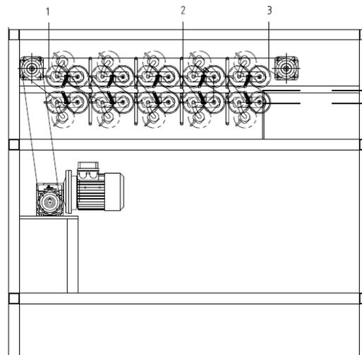
Figure 3. Schematic of Cassava Peeler.
