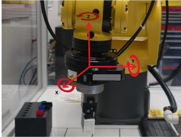
Fig. 1 Measurement of external forces and torque in six-axis using force/torque sensor
