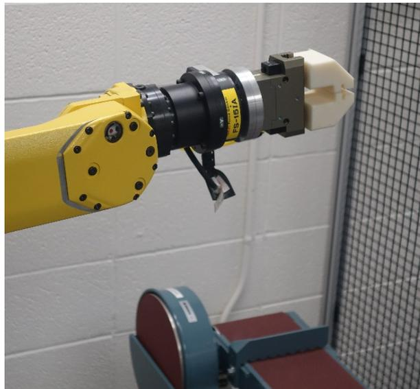
Fig. 2 Robotic arm equipped with six-axis force/torque sensor for grinding and polishing in a work cell
