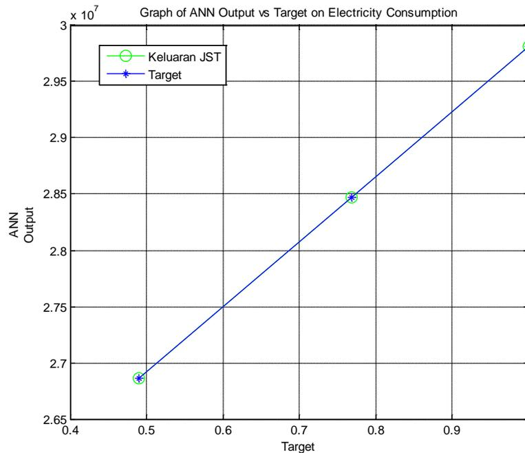
Figure 6. Graph Of ANN Output Vs Forecasting Target Of Electricity Consumption
