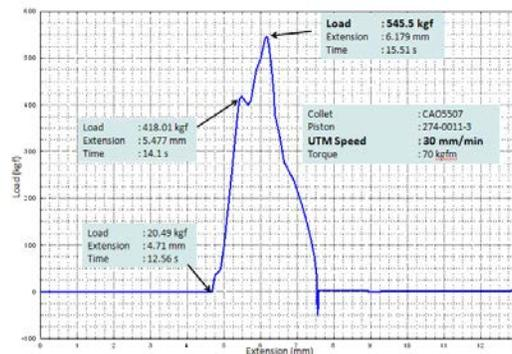
Fig 14: "Pull Load vs Stroke" plot for 30 mm/min
