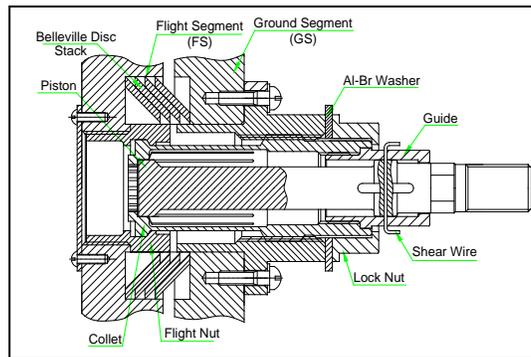
Fig.10. Test set up with Belleville disc pack
