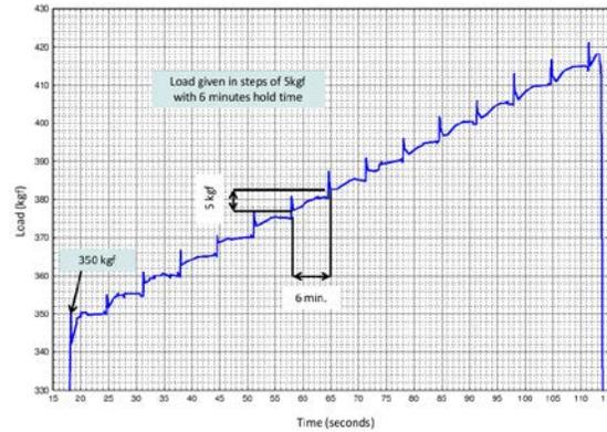
Fig 16: Close up view of gradual loading region
