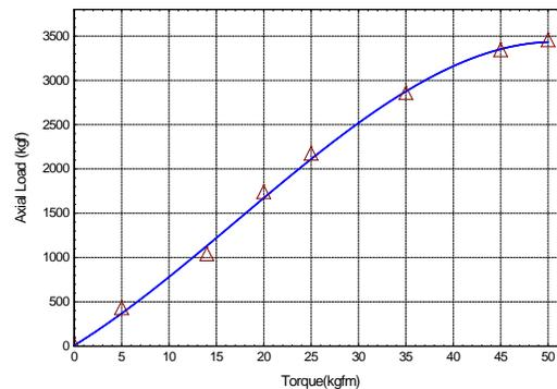
Fig 11: "Torque vs Axial Load" plot for galling
