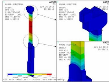
Fig 7: Equivalent Plastic Strain (Case-1)
