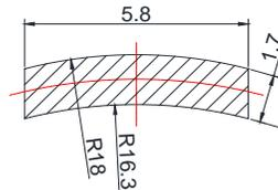
Fig.5 Cross section of collet beam
