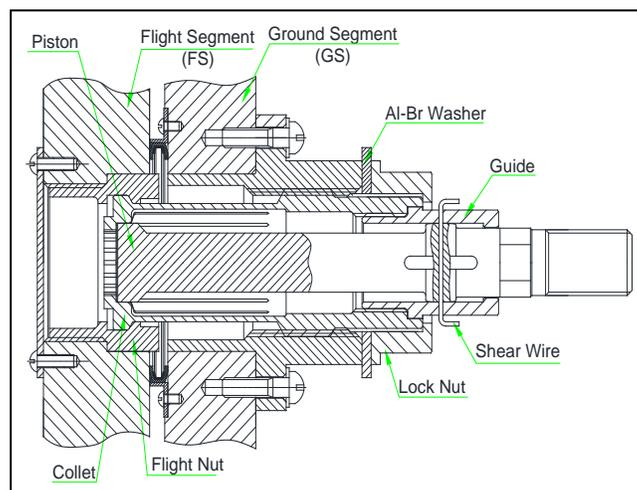
Fig.2 Collet lock configuration
