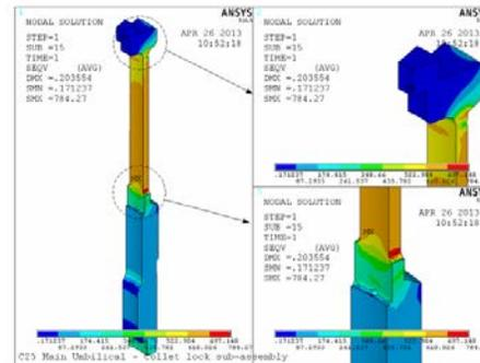
Fig 8: Von-Mises Stress Distribution (Case-2)
