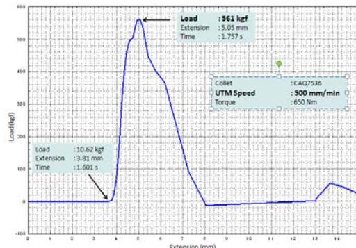
Fig 13: "Pull Load vs Stroke" plot for 510 mm/min
