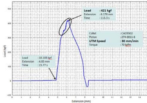
Fig 15: "Pull Load vs Stroke" plot for gradual loading
