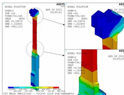
Fig.6 Von–Mises Stress Distribution (Case-1)
