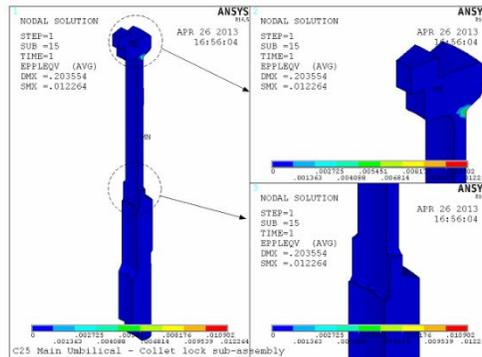
Fig 9: Equivalent Plastic Strain (Case-2)
