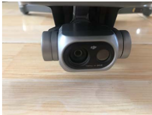
Fig. 2 The set of thermal and RGB camera
