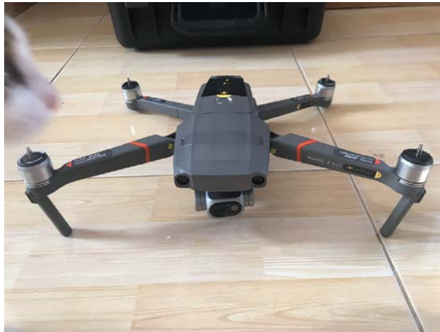
Fig. 1 Drone with thermal and visual
