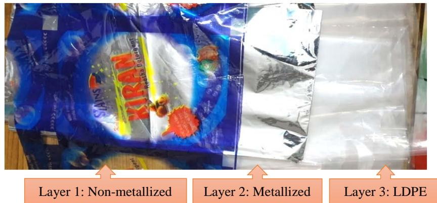
**Illustration 1: Sample of three-layered detergent pouch developed by the manufacturer**
