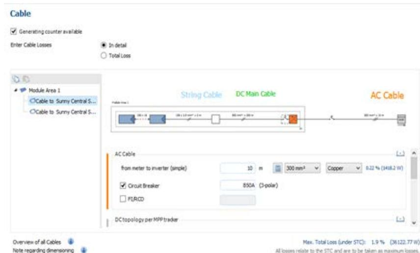
Fig. 3 The Cable diagram
