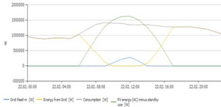
Fig. 6 The active power system on a sunny day
