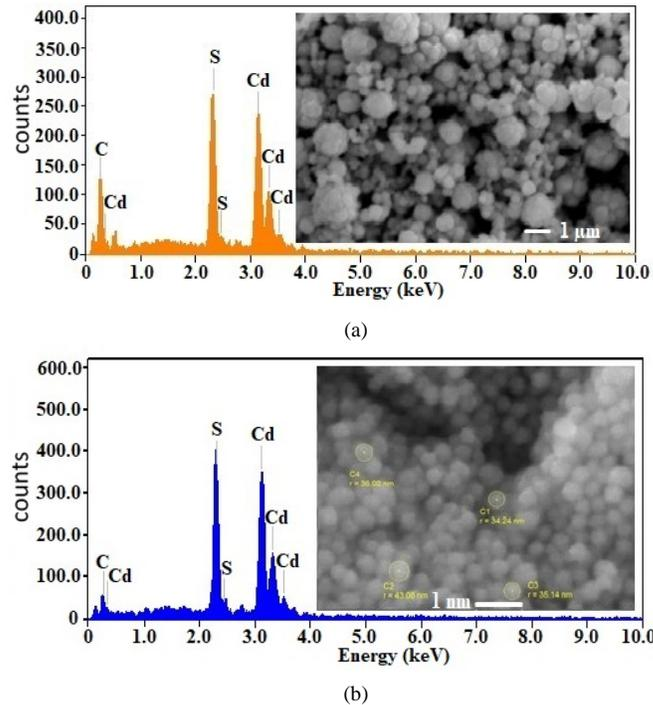
Fig. 3. EDS spectrum and SEM image (inset) of synthesized CdS nanospheres; (a) under non vacuum conditions; (b) under vacuum conditions.
