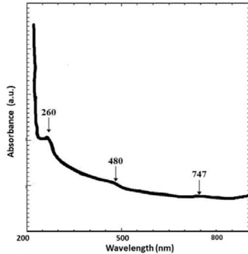
Fig. 4. Absorbance spectra of the CdS nanospheres.
