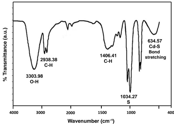
Fig. 2. FTIR spectrum of the synthesized CdS nanospheres.
