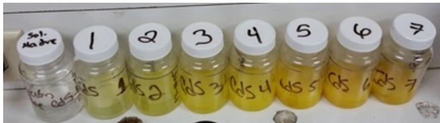
Fig. 1 Solutions heated at 140 °C for times varying from 30 to 90 min with increments of 10 min. The control (non-heated) sample is also shown.
