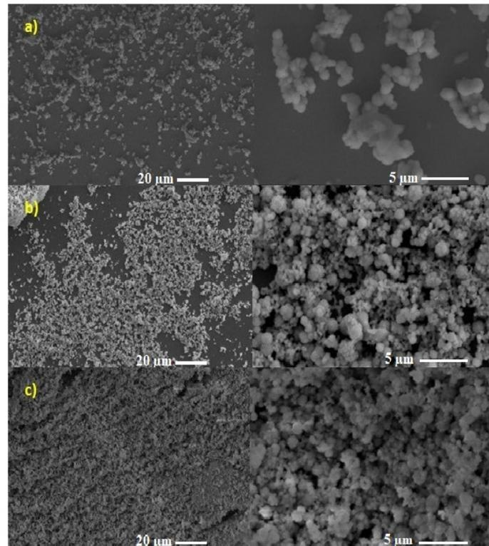
Fig. 5. SEM images of one, two and three deposited layers of CdS nanospheres after a thermal treatment of 140°C; (a) one deposited layer ; (b) two deposited layers and (c) three deposited layers.
