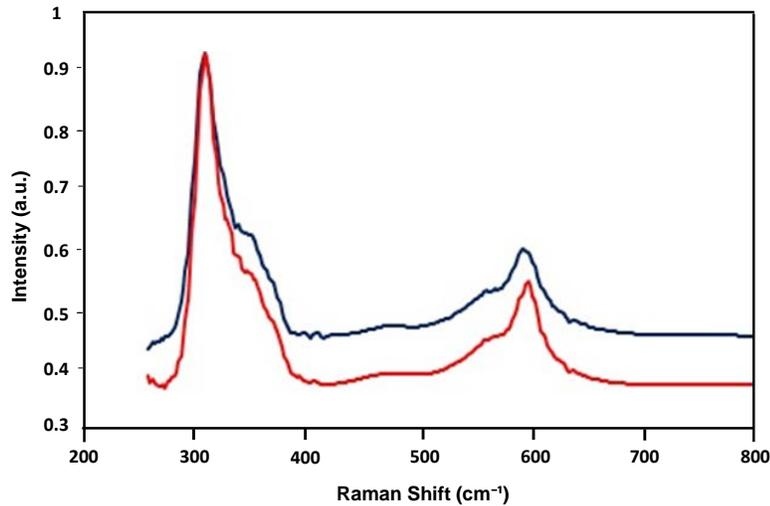
Fig. 6. Raman spectra of the sample with three CdS nanospheres deposited layers before and after the annealing process.
