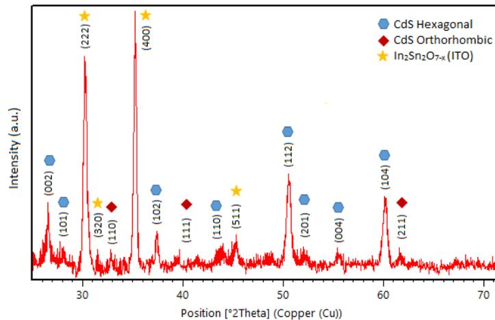
Fig. 7. CdS nanospheres thin film XRD Pattern.
