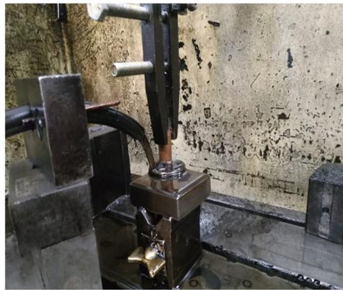
Fig 3: Placing of Electrode and Workpiece
