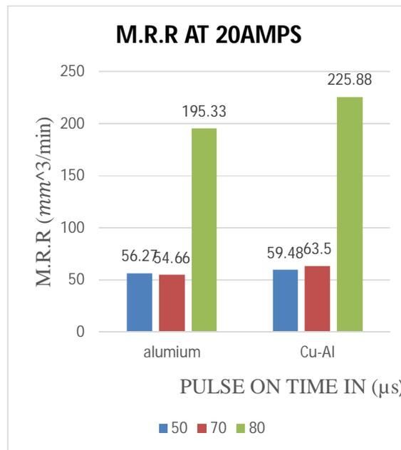
**Fig 6:** Comparative Graph of Metal Removal Rate At 20 Amps
