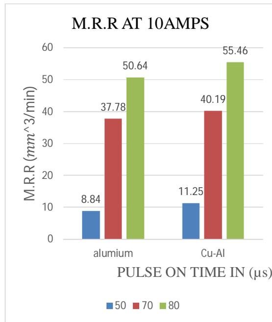
**Fig 4: Comparative Graph Of Metal Removal Rate At 10 Amps**
