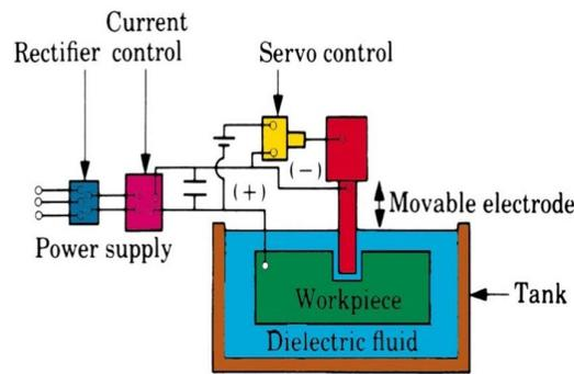
Fig 1: Setup of EDM
