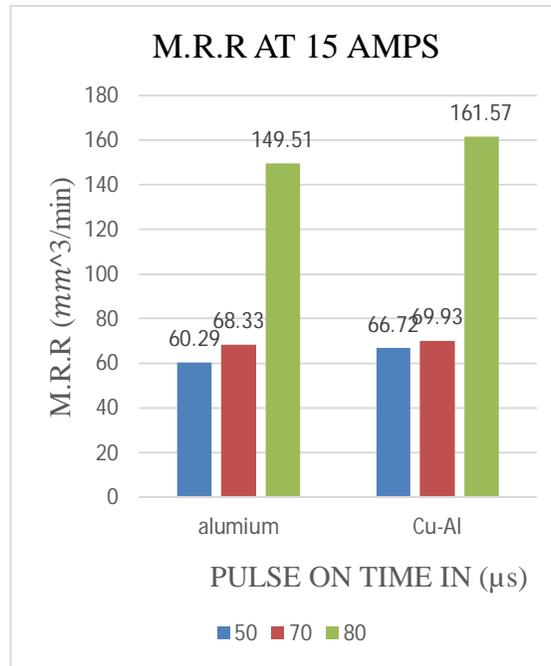
**Fig 5:** Comparative Graph of Metal Removal Rate At 15 Amps
