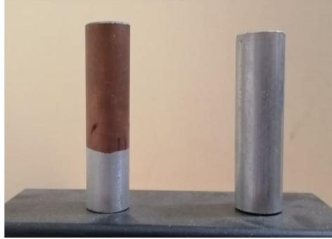
**Fig.2:** Aluminum electrode before and after electroplating
