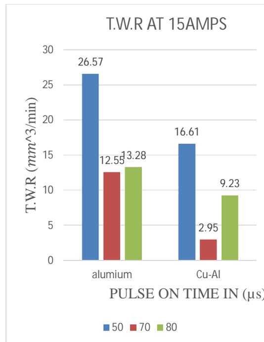
**Fig 8:** Comparative Graph of Tool Wear Rate At 15 Amps
