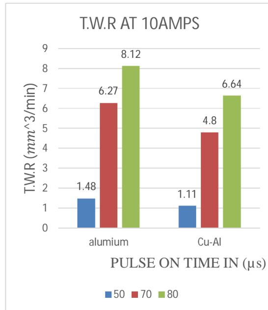
**Fig 7:** Comparative Graph of Tool Wear Rate At 10 Amps
