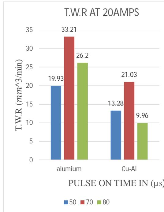
**Fig 9:** Comparative Graph of Tool Wear Rate At 20 Amps
