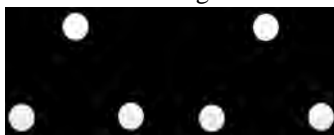
Line 1 Line 2 Fig. 3.2 Two, 3-phase Transmission lines placed side by side
