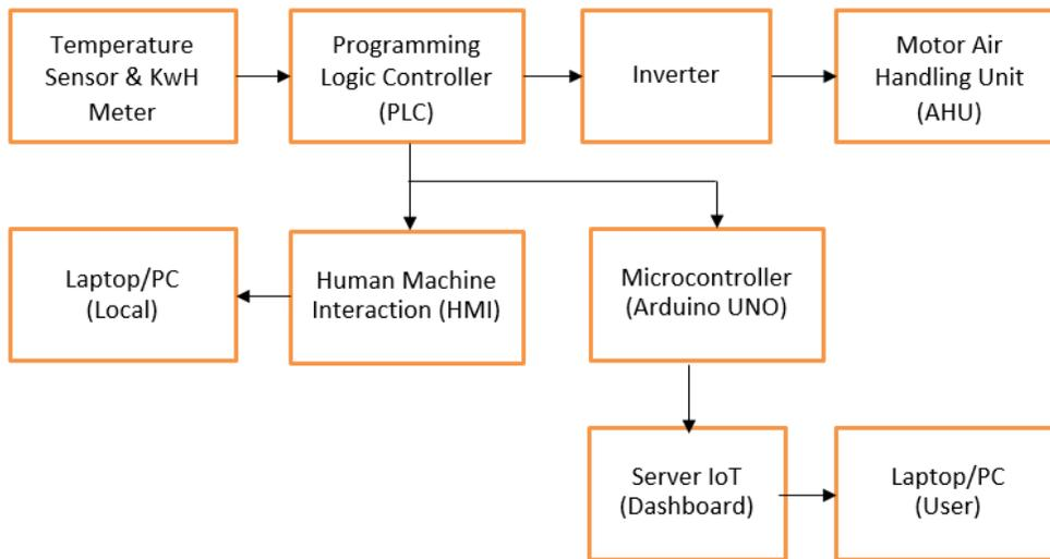
Fig 3. Diagram of the Network Topology of the AHU Machine Control System
