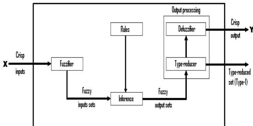
Fig.2 Structure of the Type-2 Fuzzy Inference System
