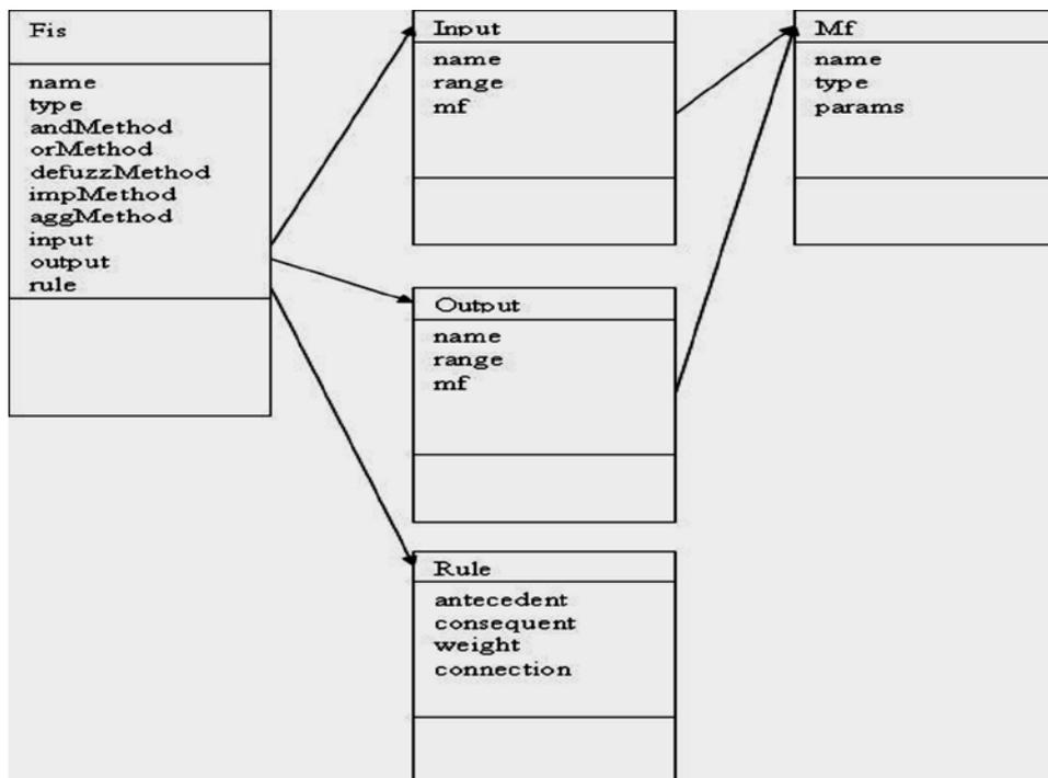
Fig.5 Hierarchy of IT2FIS structures diagram
