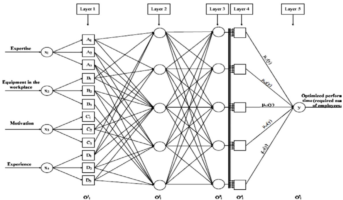
**Fig.3** A five layered feed-forward adaptive neural network for Optimization of Performance Time (OPT)
