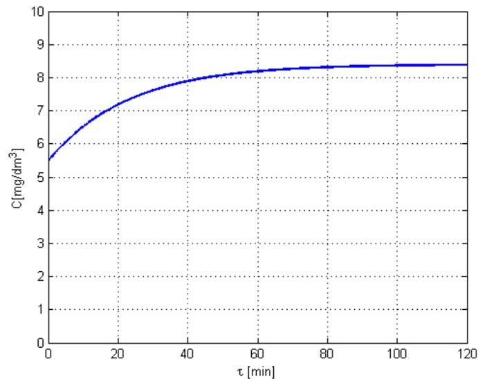
Fig. 6 Variation of the dissolved O<sub>2</sub> concentration in water as a function of time for FBG with 152 orifices Ø 0.1 mm
