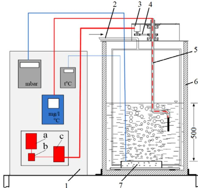
Fig. 7 Experimental installation for actuating the oxygenometer probe
