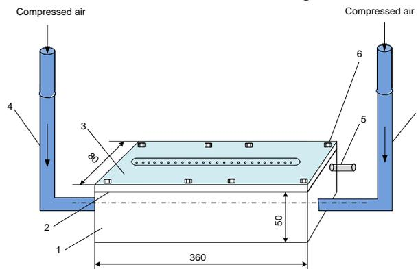
Fig. 4 Fine air bubble generator
