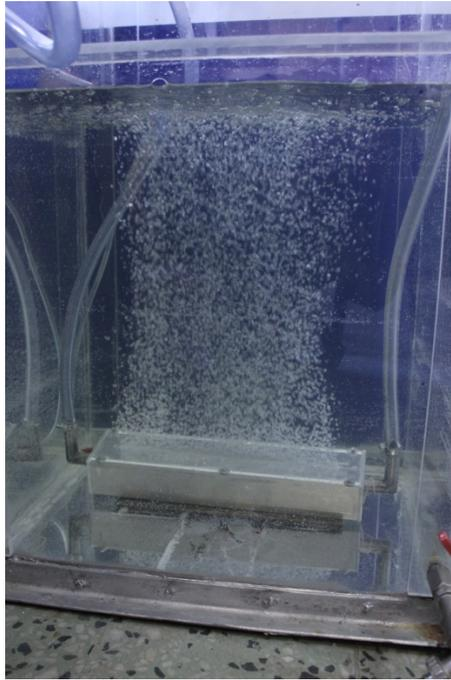
Fig. 5 Microbubble generator with 152 orifices Ø 0.1 mm in operation
