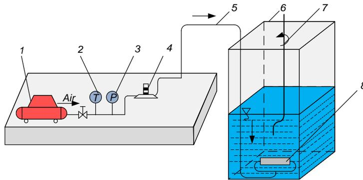
Fig. 3 Sketch of the experimental installation for introducing atmospheric air into water
