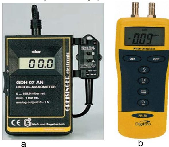
Fig. 10 Digital differential manometers.
