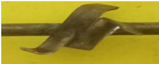
Fig 6. Angular Twisted strips of twist ratio 5.22 with opposite direction
