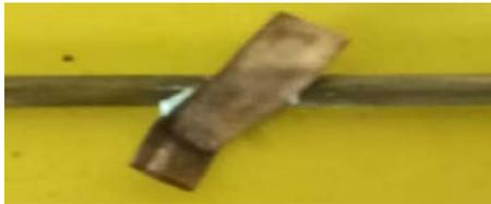
Fig 5. Angular Twisted Strips with Twist ratio 4
