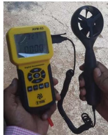
Fig 4: Anemometer
