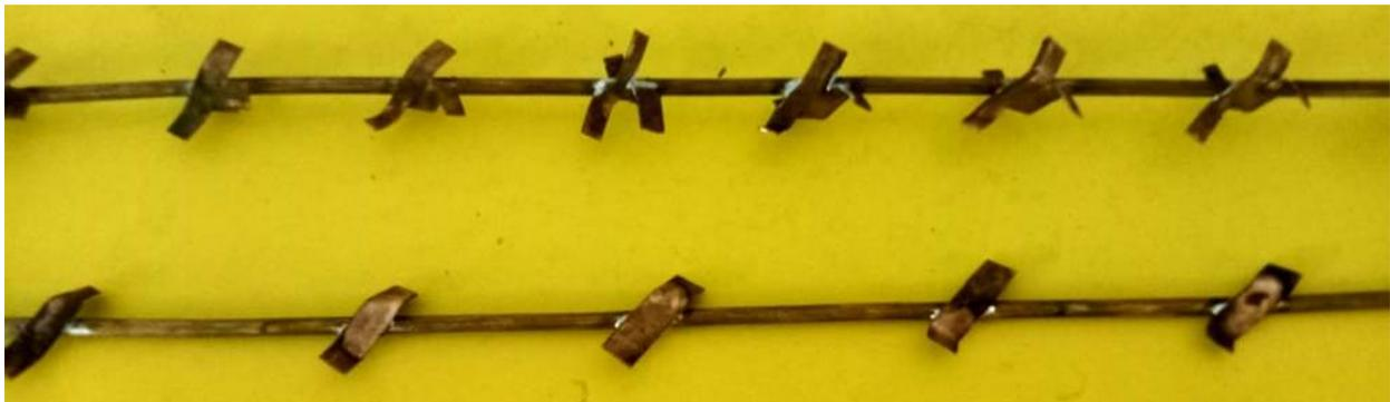
Fig 7: Angular Twisted strips of twist ratio 4, 5.22
