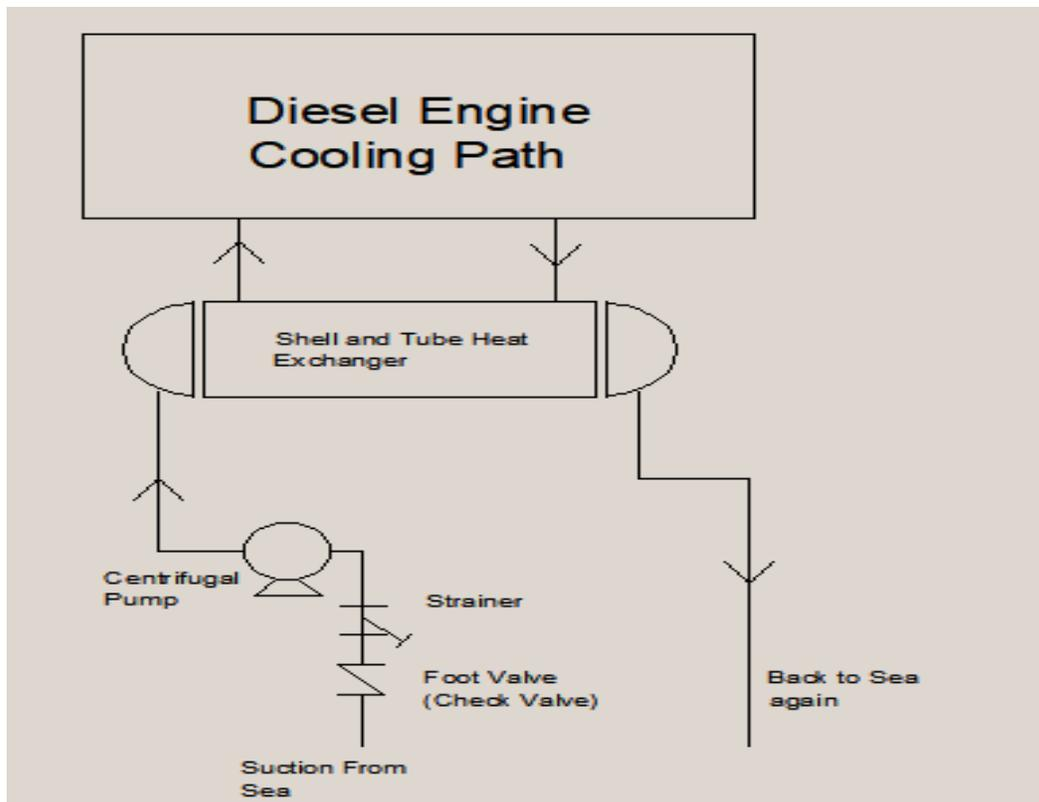
Fig. 3. Schematic drawing of Secondary Cooling Cycle
