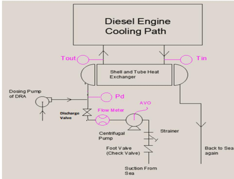
Fig. 5. DRA Dosing pump and Instruments Used
