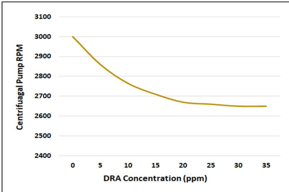
Fig. 7. Pump changing RPM with DRA concentration
