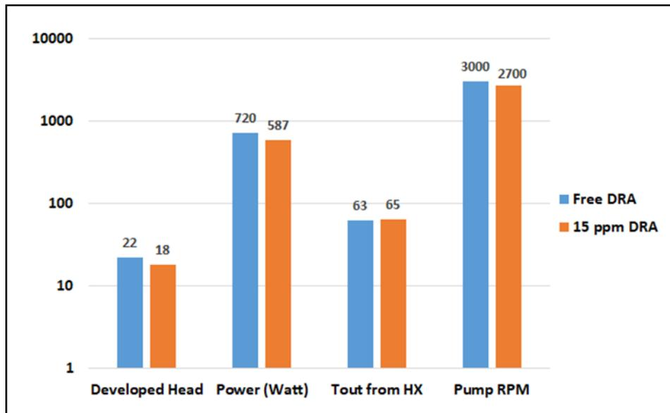
**Fig. 11. Comparison between all parameters in case of free and 15ppm of DRA**
