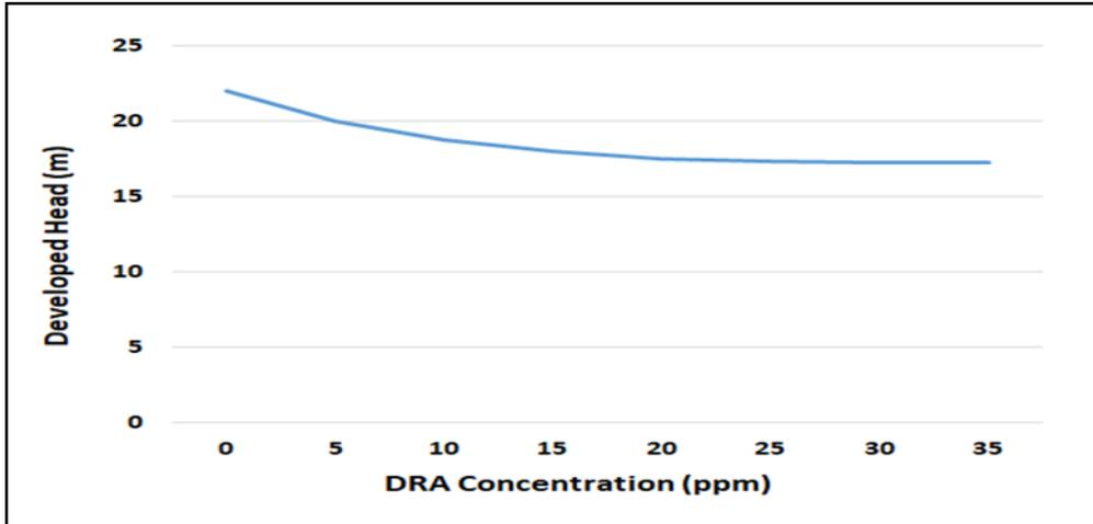
Fig. 8. Developed head changing with DRA concentration
