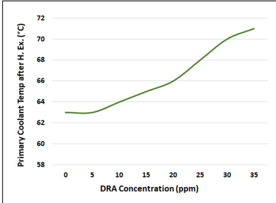
**Fig. 10. Primary coolant temperature exit from heat exchanger changing with DRA concentration**
