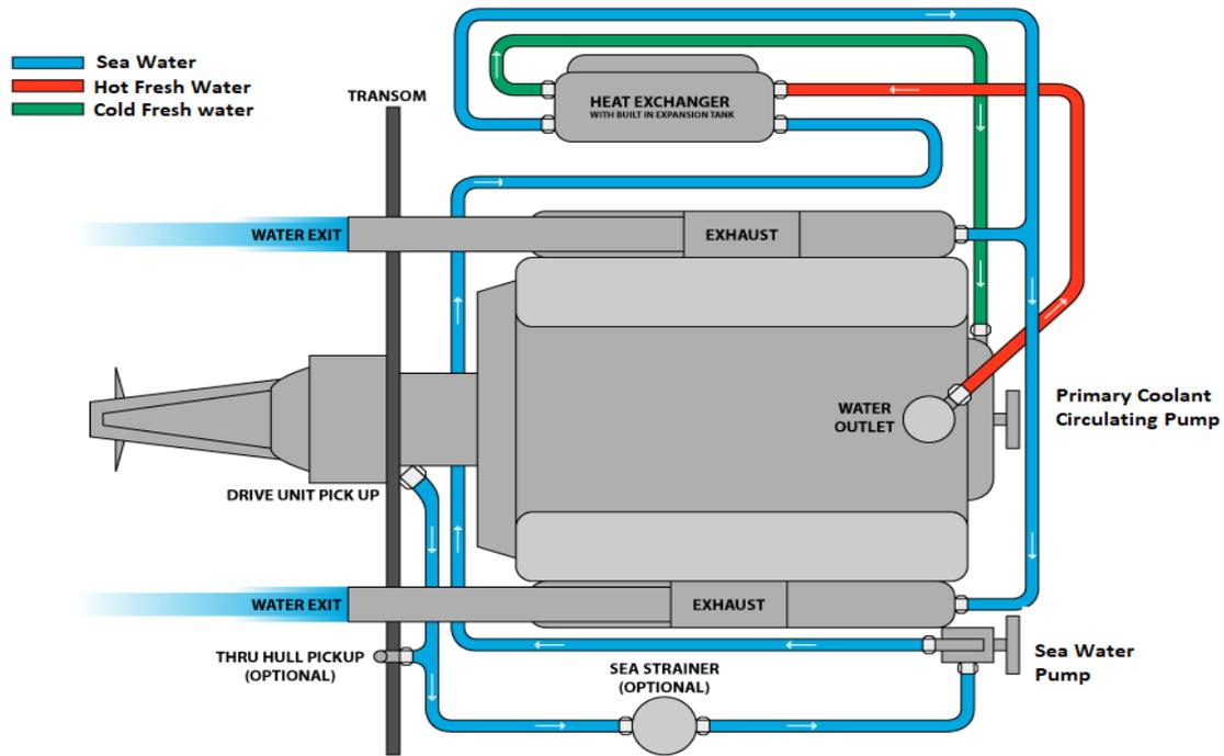
Fig. 2. Cooling Cycle for Diesel engine
