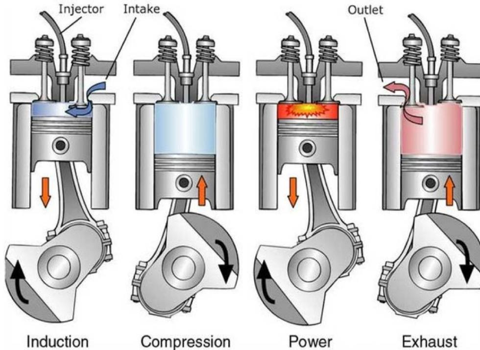
Fig. 1. Diesel engine stroking
