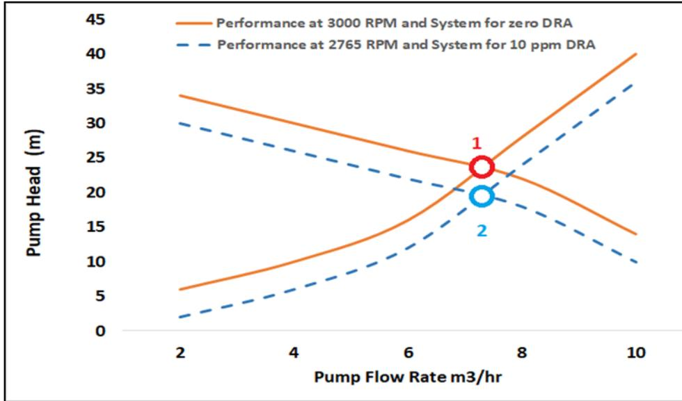
Fig. 6. New operating points at different Pump RPM
