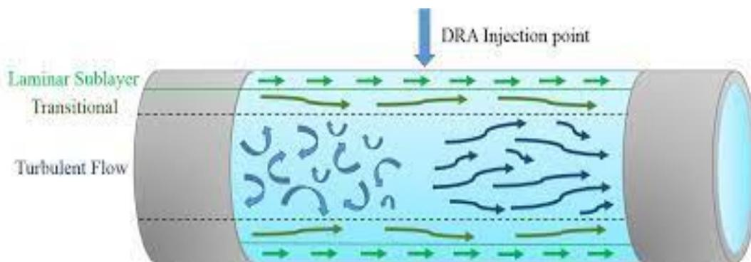
Fig. 4. DRA effect in flow turbulence reducing
