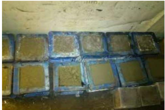
Figure 7: Concrete Cube Casted with Air Entrained SCC
