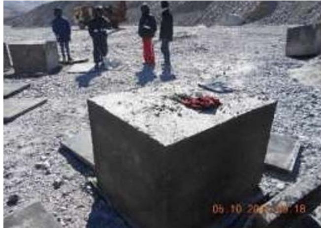
Figure 2: In-Situ Casted Cube for determining Compressive Strength
