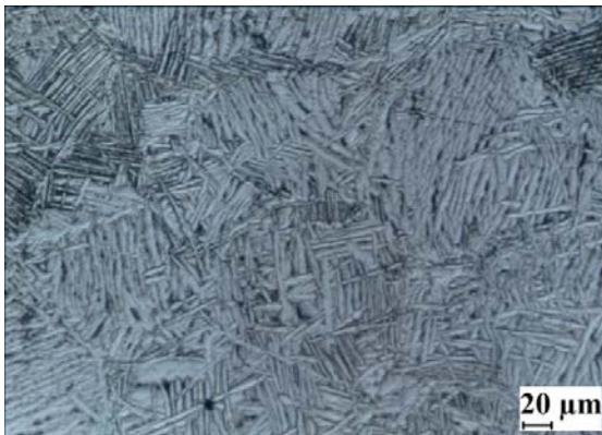
Fig. 2 The microstructure of untreated (1S) Ti-6Al-4V Alloy.
