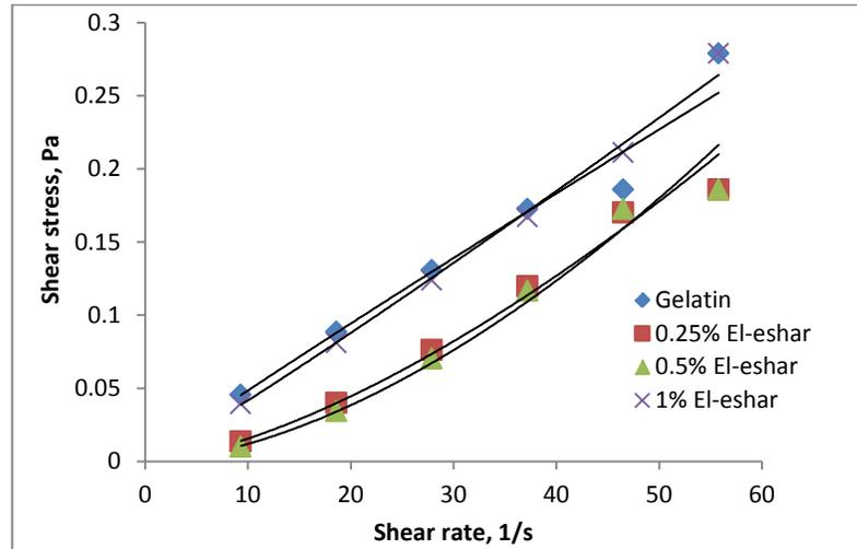
**Fig. 4. Effect of shear rate on shear stress of different edible coating blends**
