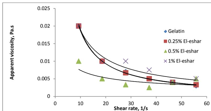
**Fig. 3. Effect of shear rate on apparent viscosity of different edible coating blends**
