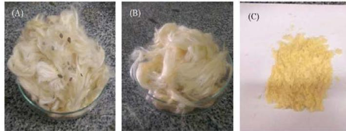
**Fig.1. (A) *Calotropis Procera* fiber, (B) Removal of seed (C) very fine particles of *Calotropis Procera* fiber**
