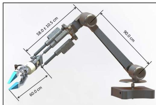
Figure 3: Dimensions of Manipulator
