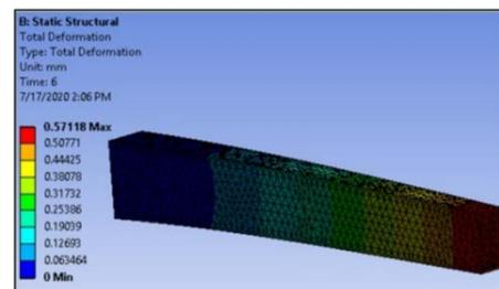
Figure 2: Deformation Analysis of Arm Links
