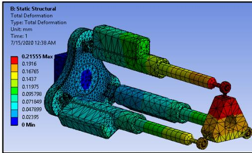
Figure 4: Analysis of Actuated System
