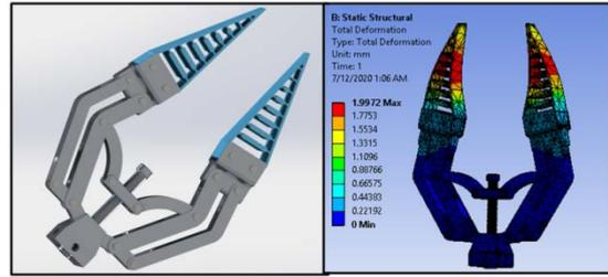
**Figure 6: Design and Analysis of Gripper**
