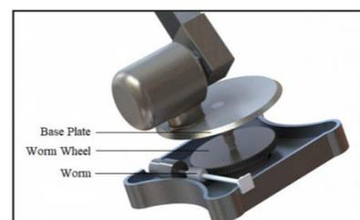
Figure 1: Base of the Manipulator
